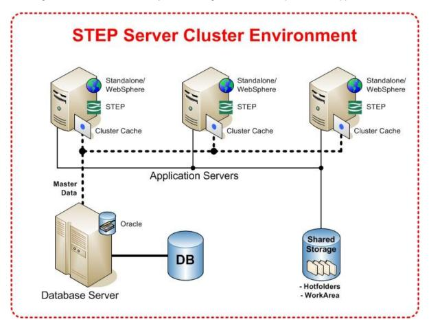
The Application Servers are physical servers running either standalone (using Oracle Java) or a WebSphere Server. Within each of the application servers an instance of the STEP Enterprise application is running supporting all three types of clients mentioned earlier (STEP Workbench clients, Web clients and DTP clients). Each application server computer has a cache of its own that is synchronized whenever write operations take place.
